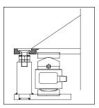
If the mount does not offer uplift protection, one may be established externally as per the drawing opposite. The uplift protection should be adjusted with a clearance of at least 1 mm and requires regular inspection of this clearance.
